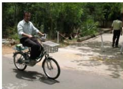
Fuel cell powered bicycle, using commercially available components
