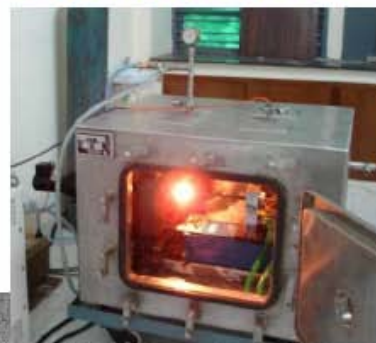
Modified Arc Discharge method for synthesis of Carbon Nanotubes
